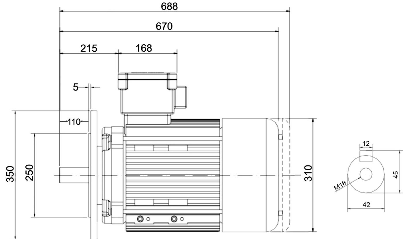
Abmessungen in mm
